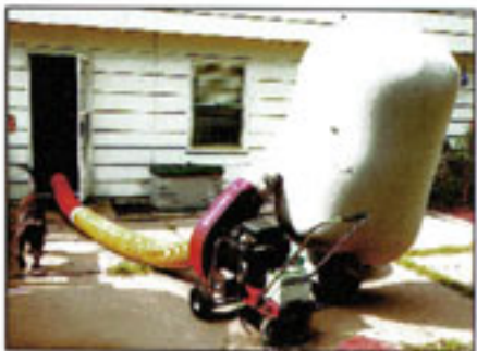
John Matus/Kansas City (Mo.) Star Cleaners say they can vacuum three grocery bags of debris from the ducts of a 2,000-square-foot home.
